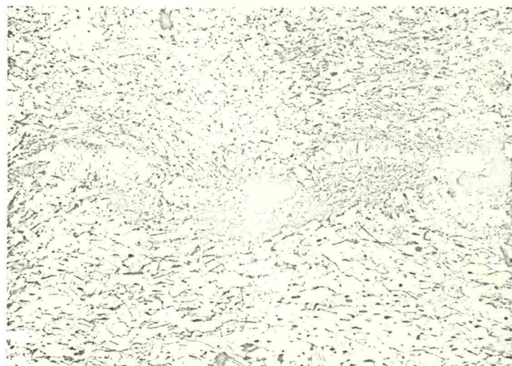
16 Continuous fusion weld in copper produced by high kinetic energy. \times 85 .
